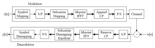
Figure 1. Block Diagram of OFDMA [10]
