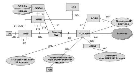
Figure 4. LTE system architecture [7]
