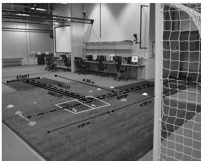
Figure 1. Experimental setup. Two 0.9 \times 0.6 m force platforms (white rectangles) are situated in the centre of the three-dimensional recording volume. Dashed line represents a sprint 90^\circ cut (90CUT), solid line represents a sprint 180^\circ cut (180CUT) and dashed-dotted line represents a sprint with quick deceleration (STOP). 90CUT, 180CUT and STOP tasks were performed on force platform 1. For the STOP task participants started to decelerate on force platform 1.
