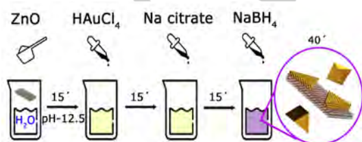
Figure 1. Simplified scheme of the reduction-precipitation steps carried out to yield anisotropic Au-ZnO nanohybrids (see Experimental for further details).
