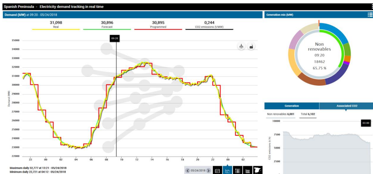
Figure 4.12: Electricity demand tracking in real time (REE, 2018).
