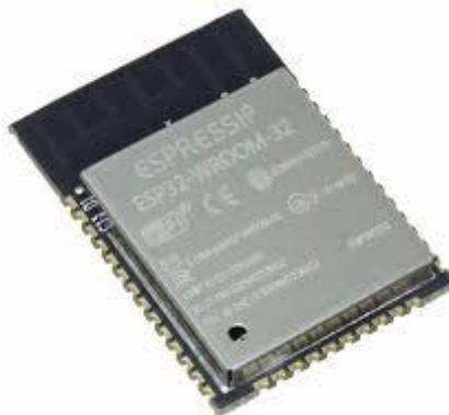
*Figura 3.2: ESP-WROOM-32 de Espressif Systems*
