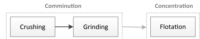
Fig. 2. Stages of modeling and simulation. The comminution process consists of crushing and grinding. The concentration is based on froth flotation.
