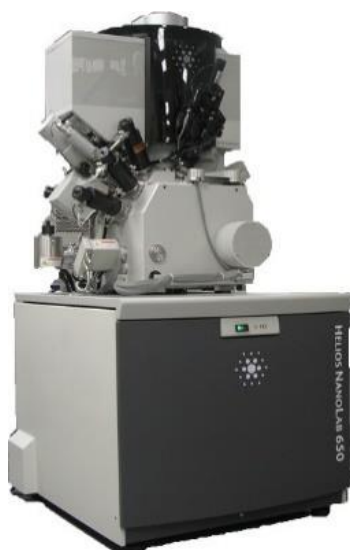
Figure 3. Photography of the FIB FEI Helios 650 used for developing these works.
