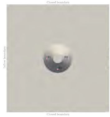
Fig. 1 Case 1. Water level probes location.
