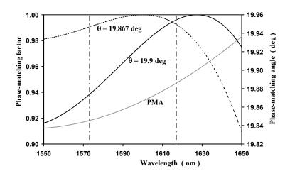
Fig 5. Phase-matching angle (PMA; grey line) and phase-matching factor as a function of the wavelength. BBO length is 2 mm. To compute phase-matching factor, two angles have been considered:  $\theta = 19.867 \text{ deg}$  (computed value at 1600 nm; dotted line) and  $\theta = 19.9 \text{ deg}$  (specified value by Eksma Optics; solid line). Dot-dashes lines delimit the spectral range of our pulses.
