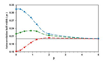
Fig 3. Autocorrelation function half-width in function of  $\beta$  for a pulse with a full width of: 0.2 ps (without dispersion; red line), 0.4 ps (chirped pulse; green line), and 1 ps (more chirped pulse; blue line).
