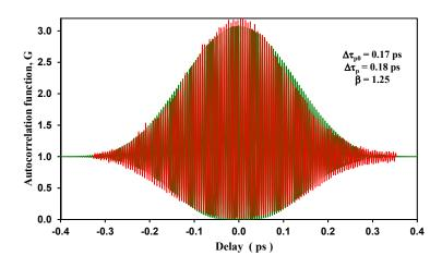
**Fig 7.** Autocorrelation trace (red line) and fitted theoretical function (green line). The temporal width of the pulse is fitted to 0.18 ps. The  $\beta$ -parameter value results 1.25. The contrast is around 3:1 instead of 8:1.
