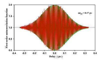
**Fig 6.** First-order autocorrelation trace (red line) and fitted theoretical function (green line). The temporal width of the Fourier-limited pulse is fitted to 0.17 ps.
