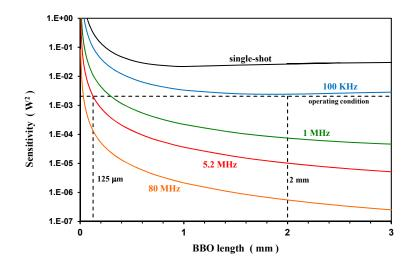
Fig 9. Autocorrelator sensitivity in function of the nonlinear crystal length for several modulation frequencies.
