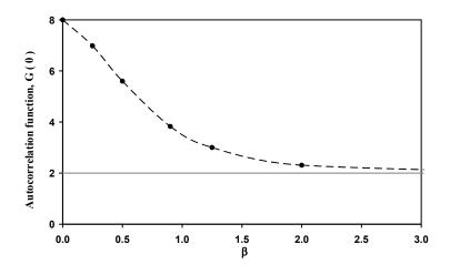
Fig 2. Maximum values of the autocorrelation function G(0) in function of  $\beta$  for a pulse duration of 0.2 ps. As the second-harmonic generation raises, G(0) diminishes and tends asymptotically to 2 (grey line), that is to say, G(0) tends to  $G_1(0)$ .
