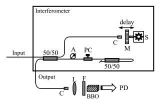
**Fig 4.** Scheme of the autocorrelator: S = servo-actuator; M = aluminium flat mirror; C = collimator (gradient-index lens); PC = polarization controller; A = variable attenuator; L = 30 mm focal length lens; F = bandpass filter (715-1095 nm); BBO = nonlinear crystal of  $\beta$ -barium borate (2 mm length); PD = photodiode (Si or InGaAs).
