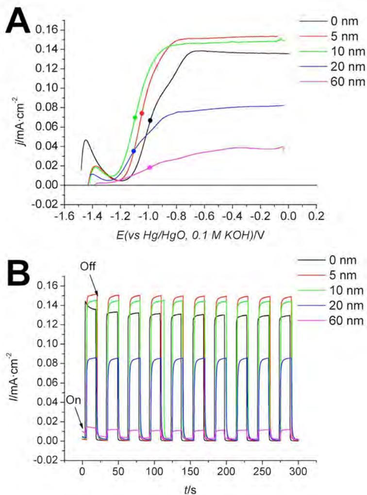
**Figure 6.** (A) Cyclic voltammograms (anodic sweep) at 20 mV·s<sup>-1</sup> under illumination and (B) chronoamperograms at 0.4 V for the TiO<sub>2</sub> and ECrGO/TiO<sub>2</sub> electrodes in 0.1 M NaOH + 0.1 M MeOH.
