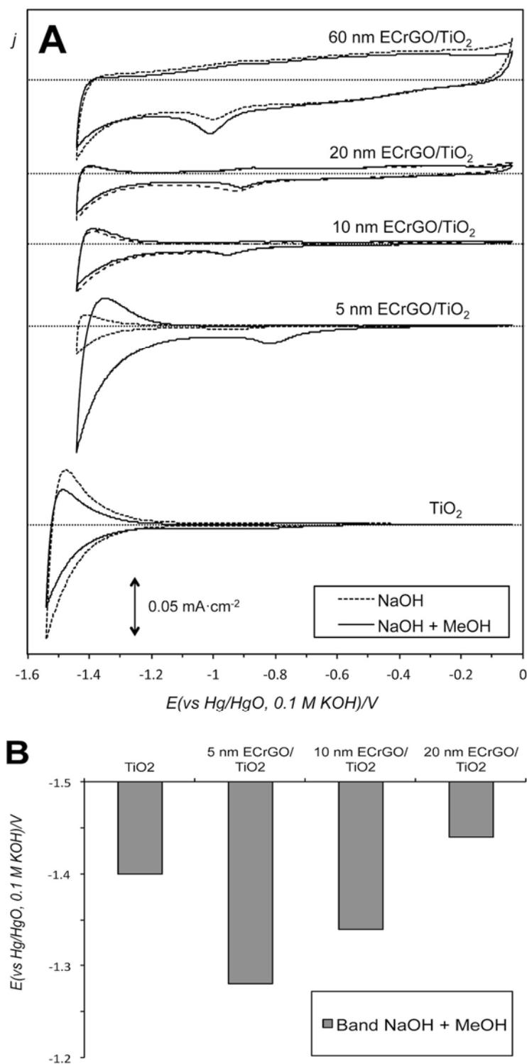
**Figure 5.** Electrochemical characterization in dark conditions for the TiO<sub>2</sub> and ECrGO/TiO<sub>2</sub> electrodes: A) Cyclic voltammetry in 0.1 M NaOH and 0.1 M NaOH + 0.1 M methanol ( $v=20 \text{ mV}\cdot\text{s}^{-1}$ ); and B) approximate position of the TiO<sub>2</sub> conduction band.
