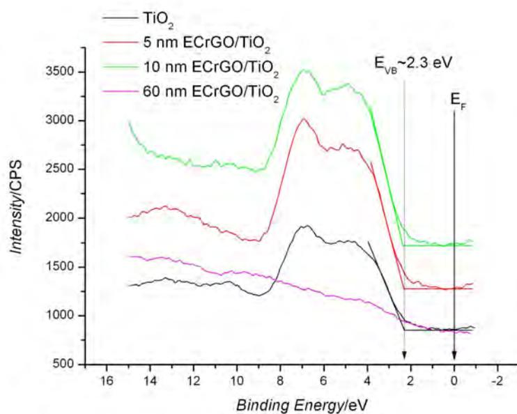
**Figure 3.** Valence band XPS spectra for the TiO<sub>2</sub> and ECrGO/TiO<sub>2</sub> electrodes.
