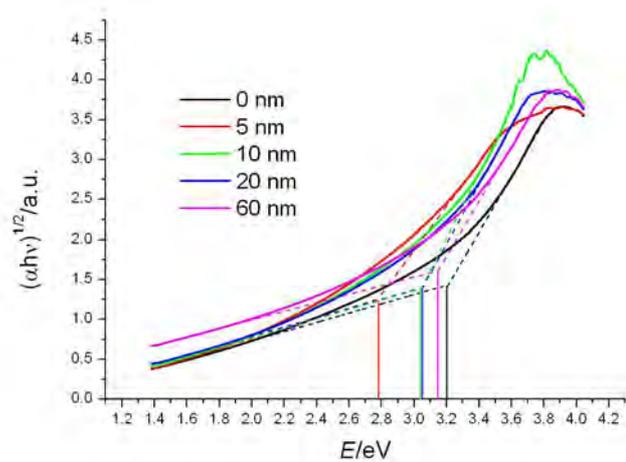
**Figure 2.** Tauc plot for the TiO<sub>2</sub> and ECrGO/TiO<sub>2</sub> electrodes.
