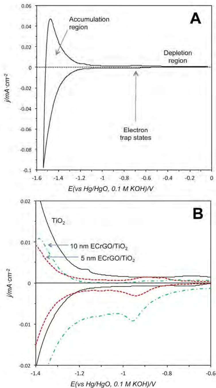
**Figure 4.** Cyclic voltammetry in dark conditions (0.1 M NaOH,  $v=20 \text{ mV}\cdot\text{s}^{-1}$ ): A) Blank  $\text{TiO}_2$  indicating the voltammogram main regions; and B)  $\text{TiO}_2$  compared to the ECrGO/ $\text{TiO}_2$  electrodes with the thinnest ECrGO films.
