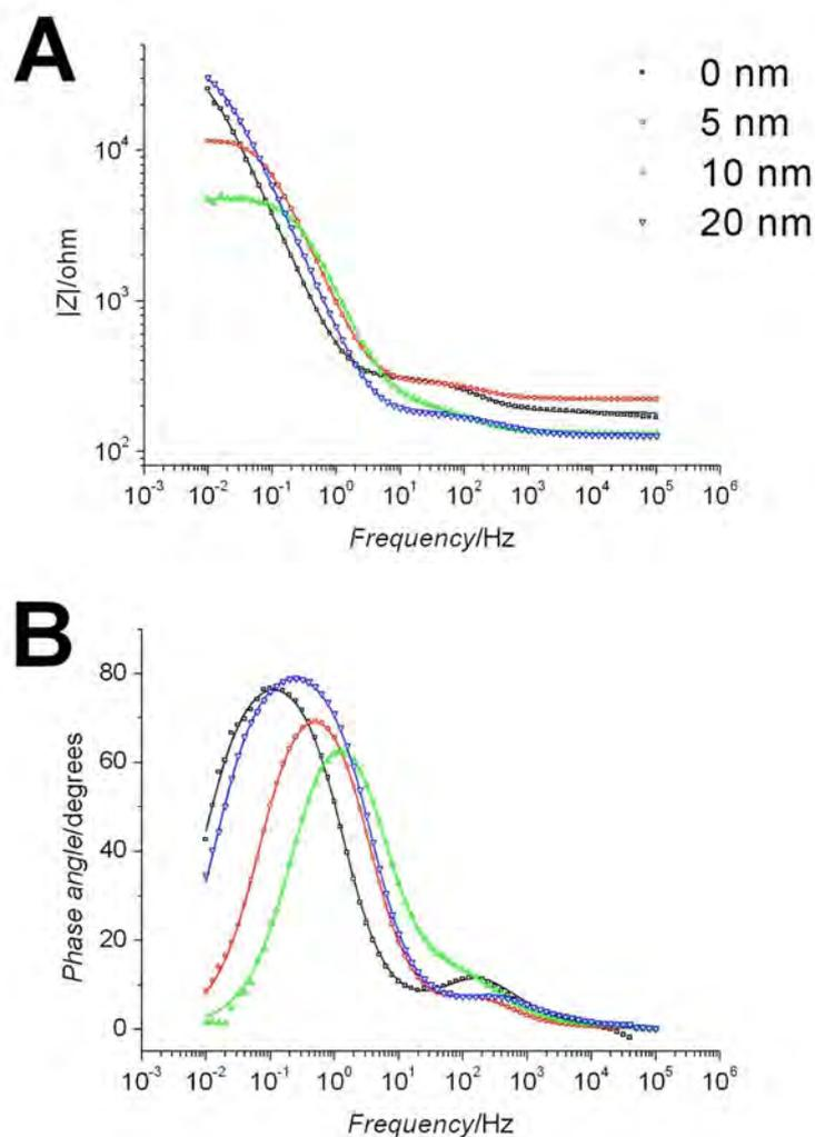
**Figure 8.** Electrochemical impedance spectroscopy for the TiO<sub>2</sub> and ECrGO/TiO<sub>2</sub> electrodes under illumination in 0.1 M NaOH + 0.1 M methanol: A) impedance modulus Bode plot, and B) phase Bode plot. Measurements were performed at the respective OCP: -1.31 V for TiO<sub>2</sub>, -1.06 V for 5 nm ECrGO/TiO<sub>2</sub>, -1.13 V for 10 nm ECrGO/TiO<sub>2</sub>, and -1.22 V for 20 nm ECrGO/TiO<sub>2</sub>.
