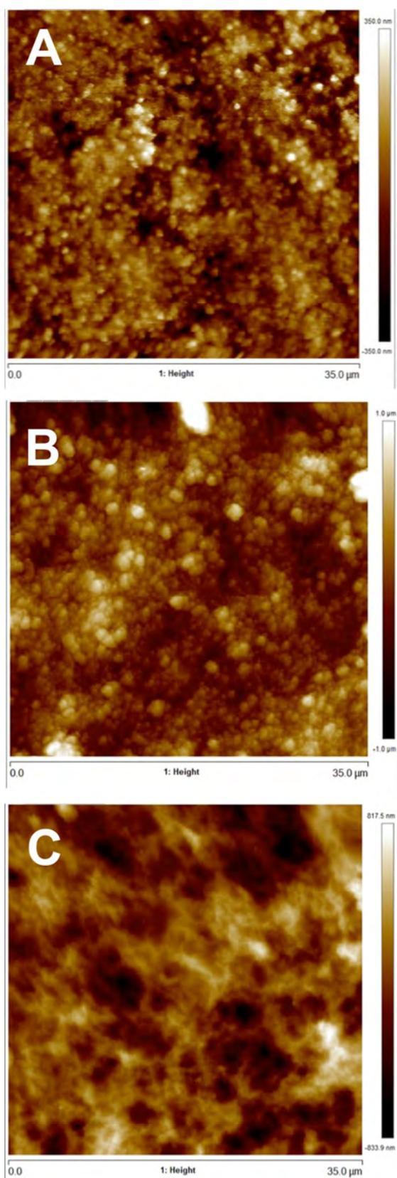
**Figure 1.** 35x35 μm AFM images of different electrodes: A) TiO<sub>2</sub>, B) 10 nm ECrGO/TiO<sub>2</sub>, and C) 60 nm ECrGO/TiO<sub>2</sub>.
