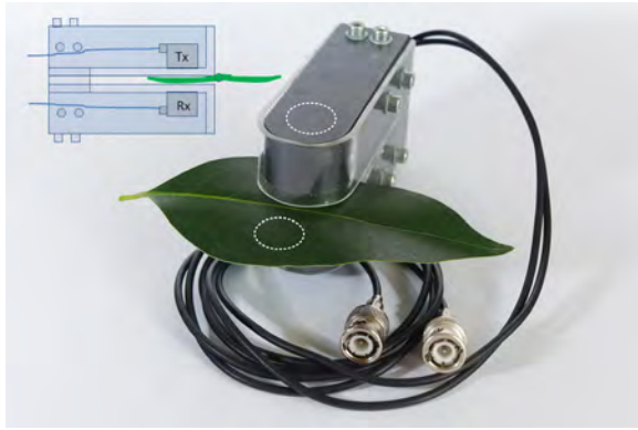
FIG. 1. Picture of the device used for the measurements: a U-shaped holder for the transducers (Tx and Rx) and a polycarbonate cover that provides a slot to properly place the leaf for the measurement. The two white dashed circle lines indicate the location of the transducer in the holder and the size and the position of the area where measurements were performed on both sides of the midrib (only one is indicated).
