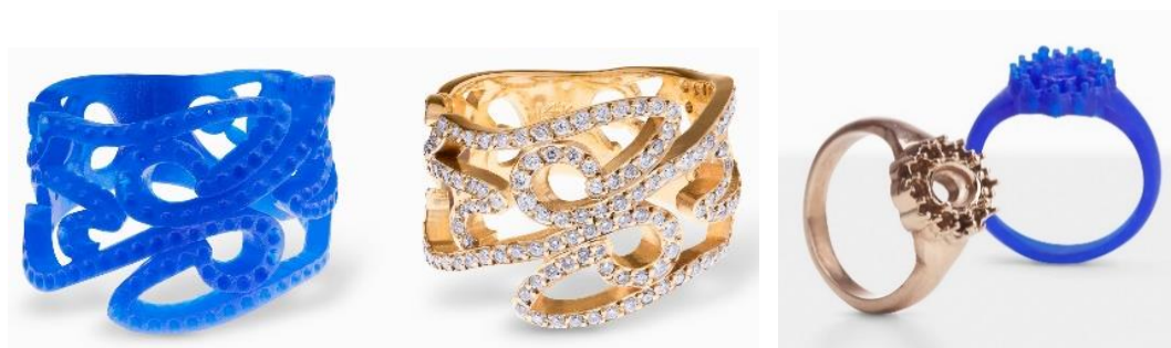
PICTURE 4. Jewelry produced by investment casting with 3D printed models.
