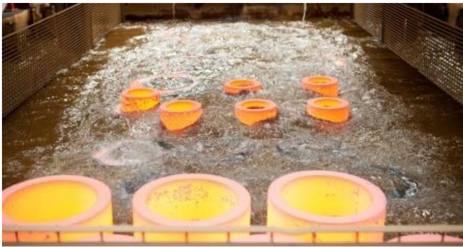
Figure 3: Industrial water tank used for quenching [5]
