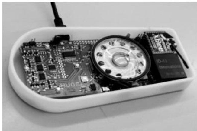
Fig. 5.24 RaPIDO device hardware (Soute et al., 2017)
