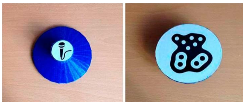
Fig. 4.19 New tangible selector to record audio in NIKVision tabletop.
