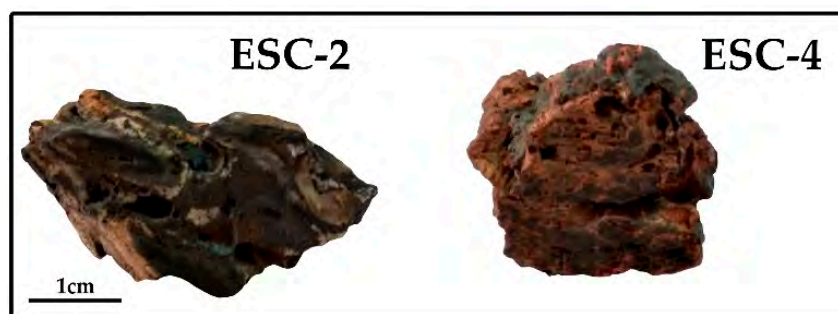
Figure 1. Images of a black natural clinker sample with yellow areas (ESC-2) and another red with black areas (ESC-4).
