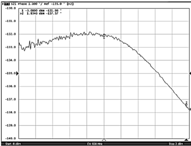
Figure 5. AM-PM characteristic of the RF5110G amplifier.
