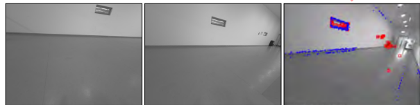
Fig. 3: [TUM monoVO] Failure recovery in sequence 40 : At t_1 and t_2 , the feature-based module fails due to the lack of features in the scene, whereas the direct module is able to track the high-gradient pixels. At t_3 , the scene now contains a sufficient number of features, and their depths can be initialized with the help of the direct module.
