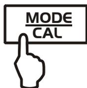
⇒ Remove all loads from the balance and press repeatedly the **MODE** key until „PtArE“ flashing appears.
