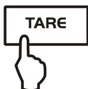
⇒ Unload the balance and press the **TARE** button, the zero display appears.
