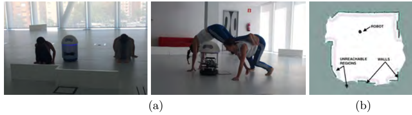
Fig. 4. (a) Images from training sessions where we can see the panels used to limit the robot map of the performance space. (b) Sample map from the performance area.
