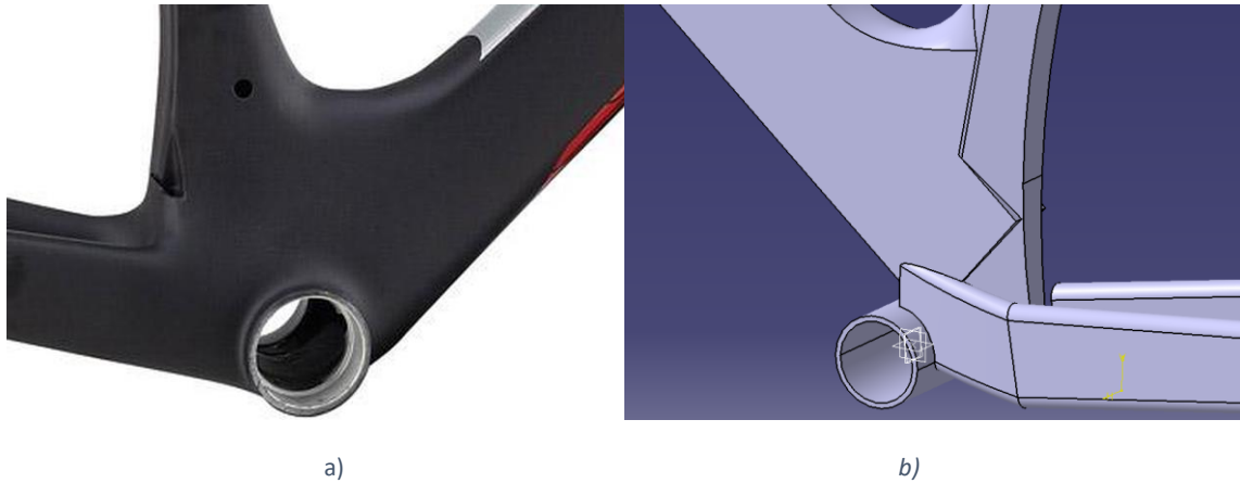
Figure 7: Axis zone of Giant Propel Advanced in: a) Reality (H2Gear, 2018). b) CATIA V5®.
