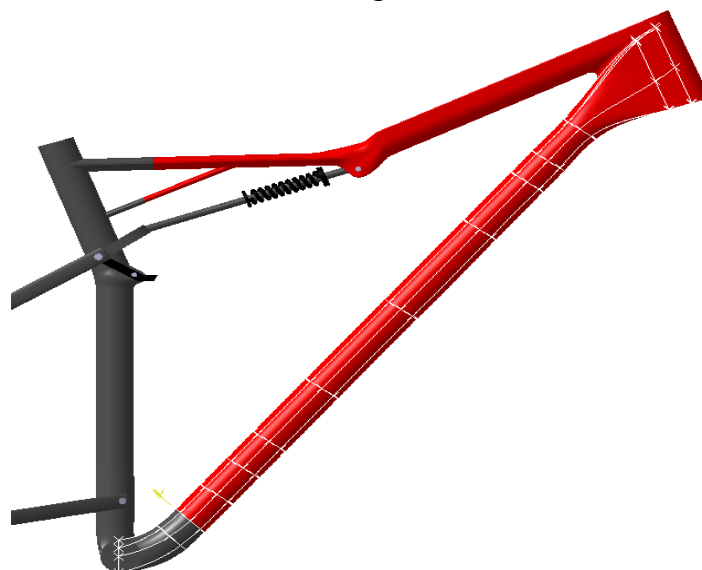
Figure 28: Diagonal tube geometry sketch.
