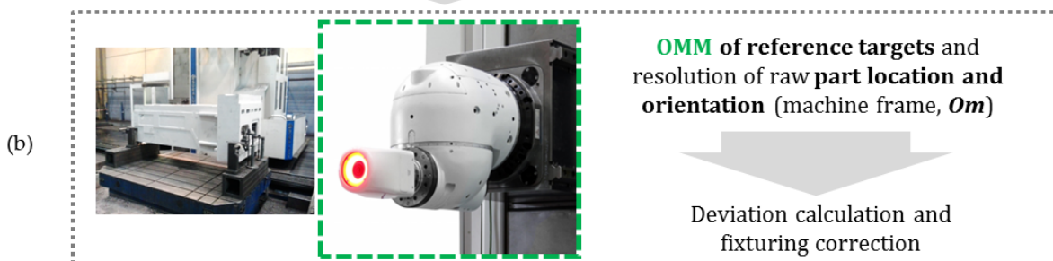
71 Figure 1. Vision OMM system for raw part alignment in milling. (a) Out-of-machine raw part 72 measurement by portable photogrammetry and fitting to ideal CAD geometry. (b) On machine 73 stereo-photogrammetric vision system for raw part location and orientation measurement.
