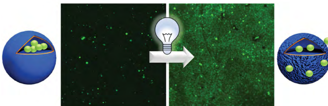
Figure 1.6 Confocal fluorescence microscopy images showing the light stimulated release of Rhodamine B upon UV irradiation of loaded vesicles.
