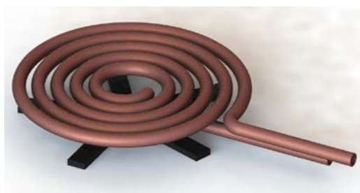
Fig. 1. Schematic representation of a power pad with tubular conductor..
