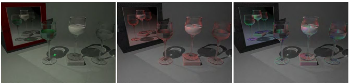
Figure 3: Cups scene, depicting a scene with a dielectric mirror, and a set of glass cups filled with absorbing, scattering and a non-participating dielectric media. From left to right: radiance, degree of polarization and orientation of linear polarization. The scene shows the slightly polarizing effect of very scattering and optically thick media, specially visible in the middle cup.
