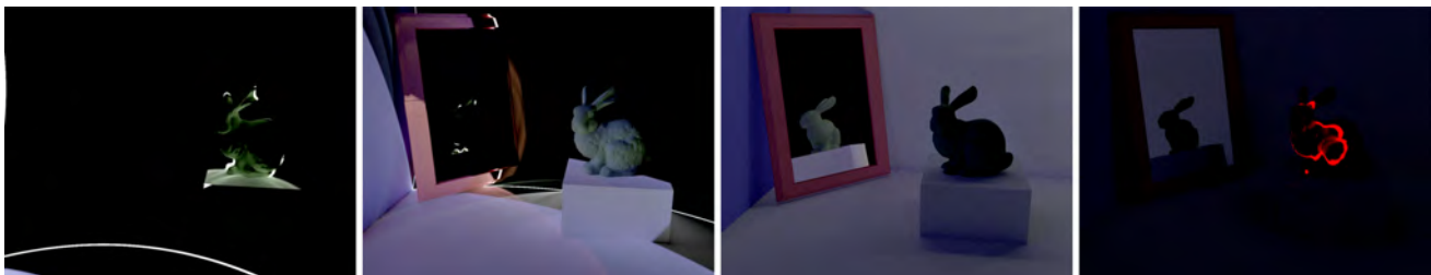
Figure 6: Time-resolved render for the bunny scene: From left to right, light travels from the light source to the bunny, which reflects most green light and absorbs red and blue light. Note that this reflection before reradiation would be the result if a scalar version of the algorithm was used. Light continues propagating, illuminating the scene via multiple reflections, while the mirror starts reflecting the bunny. After several diffuse reflections, light loses its directionality, becoming mainly diffuse lighting. Finally, after a few nano-seconds, absorbed light is re-emitted by the fluorescent bunny red-shifted. We refer to the supplemental video for the full animation.
