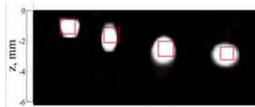
Fig. 2. Black and white representation of the normalized heat source distribution retrieved from experimental data obtained for different depths of a 1 x 1 mm square Cu slab. Real contours in red.
