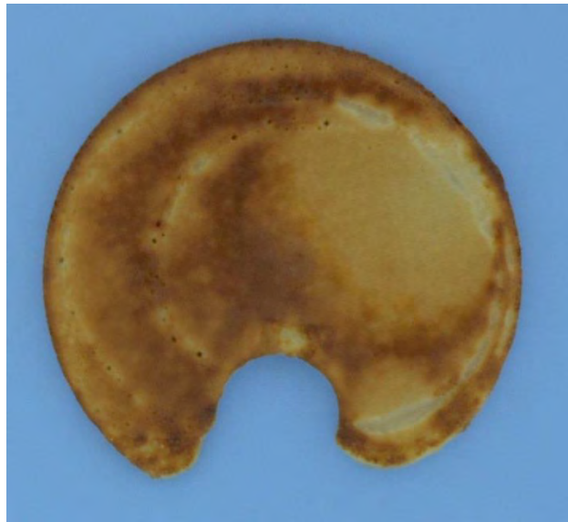
Fig. 6. Picture of a pancake cooked using a set temperature of 240°C during 180s in the uniform-heating rig. Images scale is 380 pixels per inch, the color space is sRGB.
