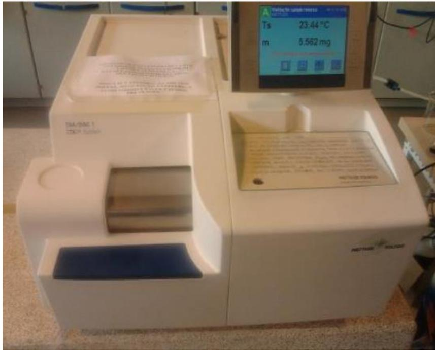
Figura 33. Mettler Toledo TGA/STDA 851e.
