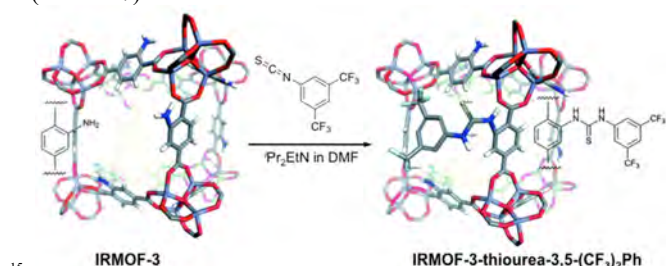
Scheme 7 PSM approach between IRMOF-3 with 3,5-bis(trifluoromethyl)phenyl isothiocyanate. Adapted with permission from ref. 56. Copyright © Royal Society of Chemistry.
