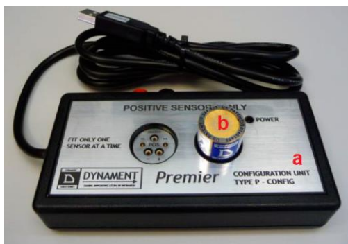
Figura 7. 8. Componentes sensor Dynamet. (A) Configuration Unit, (B) sensor
