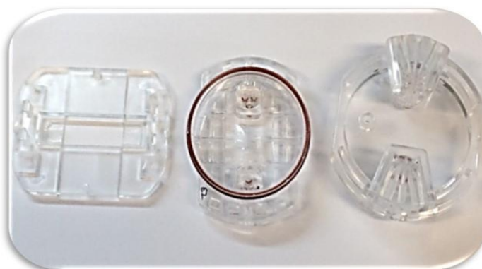
Figure 4.9: Methacrylate encapsulates. On the left is situated the piece where the fluidic device was fit. The piece in the middle of the picture closed the piece explained before. The encapsulated is completely hermetic when the piece on the right closes the other two pieces.
