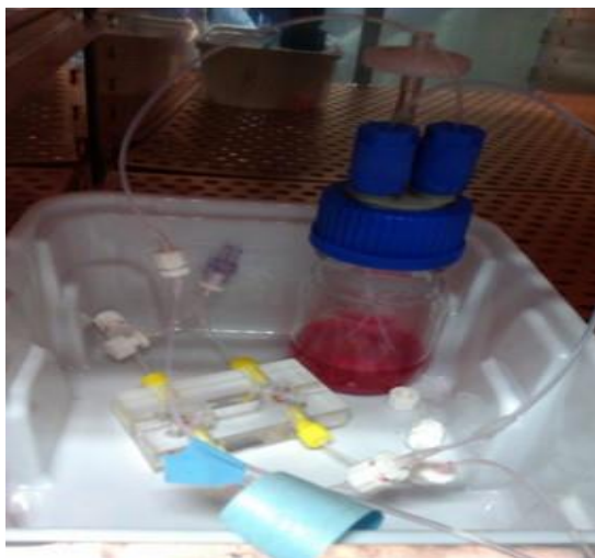
Figure 4.8: First holder prototype with two screwed pieces
