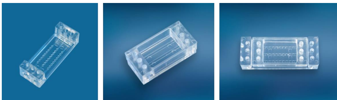
Figure 2.23: Image prototypes for the COP microdevice developed from the SU-8 prototype. Left- The bottom piece entails three arrays of microwells connected by a microchannel. Fluidic ports are placed in both ends of the microdevice for an easier liquid handling. Middle- The top piece comprises three microchannels intended for coupling fluid flow on top of the bottom piece microwells, but it can also be used to diminish reagent volumes substantially. Right- The microdevice resulting from integrating both pieces is shown.
