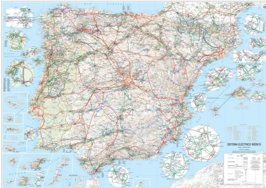
Figure 9.1. Spanish transmission grid, REE.
