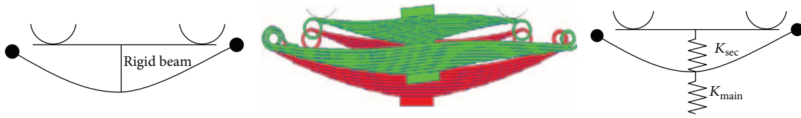
FIGURE 17: Some models of the spring for a double spring suspension.
