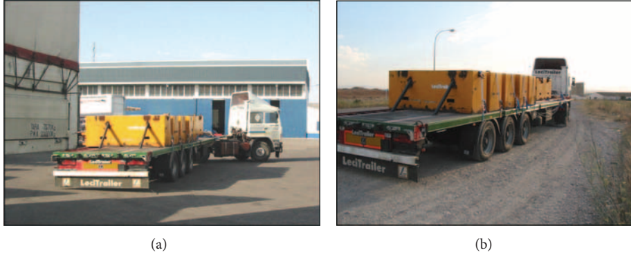
FIGURE 22: Extensometric test performed in a three-axle semitrailer.
