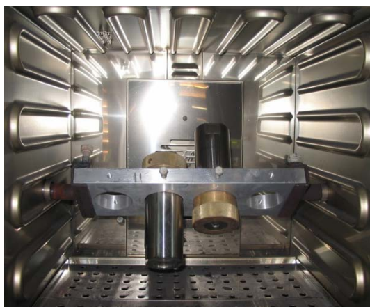
Figure S2. Picture of the rotatory oven used in the catalytic conversion of sugars reaction.
