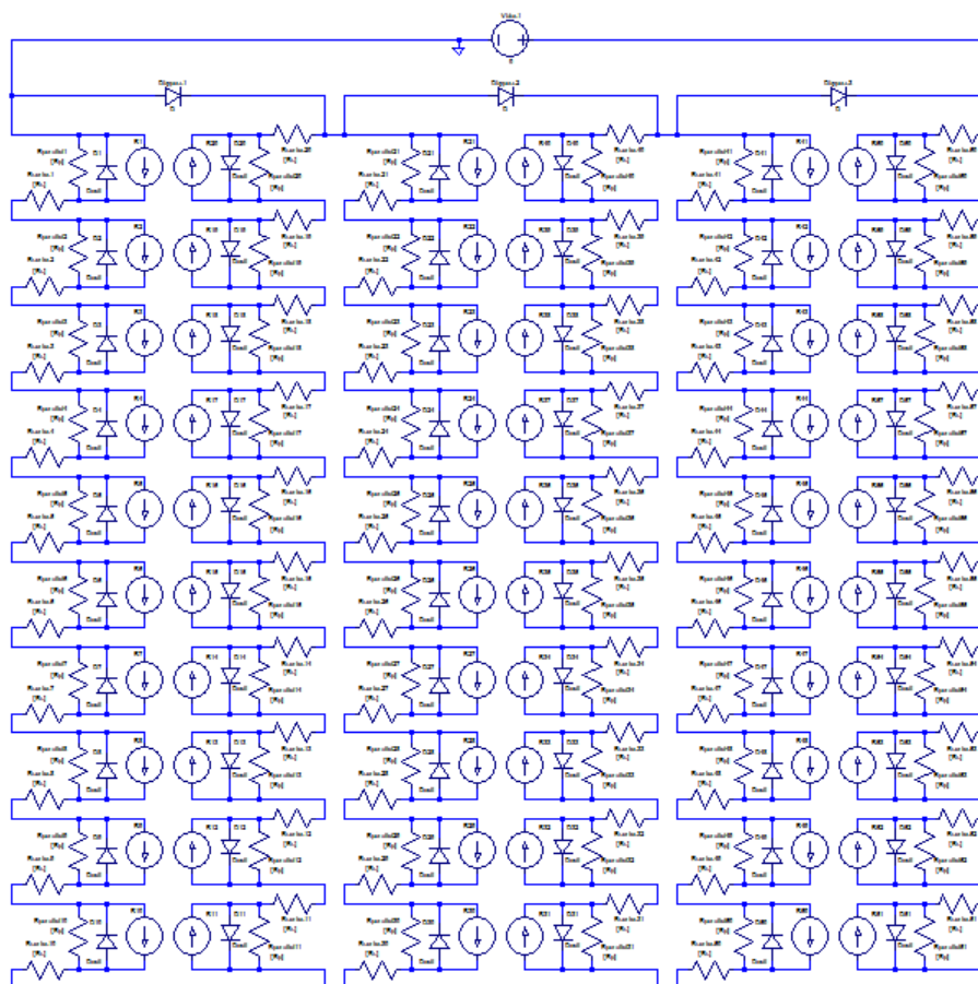
Figure 28: HIG laboratory module modelled with LTspice IV
