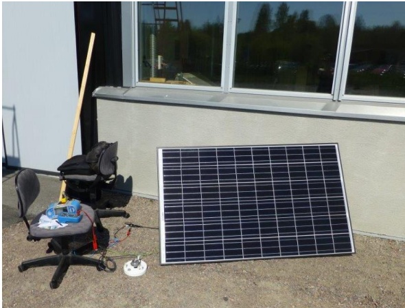
Figure 37: Windon module assembly during the base case experimental measurements at HIG laboratory
