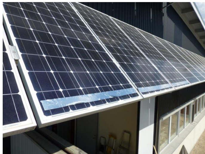
Figure 30: Case 1.3 of study (37% of a row shaded in three modules)
