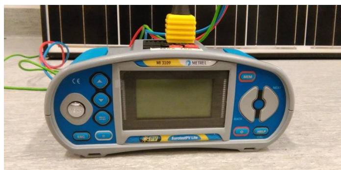
Figure 29: METREL I-V tracer EurotestPV Lite MI 3109
