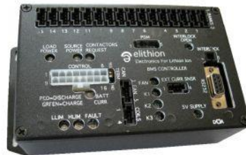
Figure 1. Lithiumate Pro. Taken from Elithion
