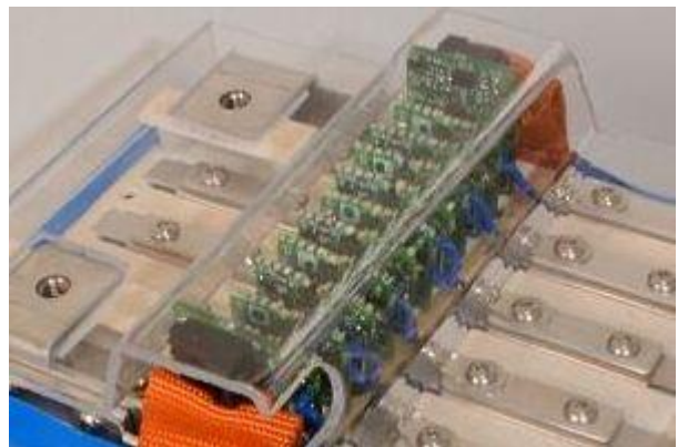
Figure 2. Slave Boards. Taken from Elithion
