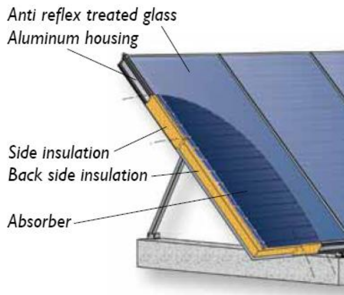
Figure 6.5: Solar collector description (Arcon, 2013)
