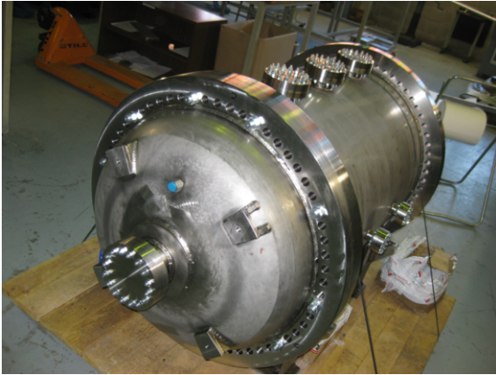
Figure 1: The NEW pressure vessel (NPV).
