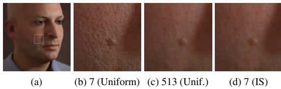
Figure 11: The quality of the rendered images, with and without importance sampling of the approximated kernel. (a) Initial image; (b) Uniform sampling with only seven samples leads to obvious aliasing artifacts; (c) Ground-truth created by uniform sampling with 513 samples; (d) Our importance sampling with as low as seven samples.
