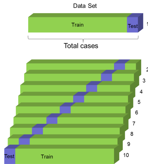
Figure 5.6: Illustration of a k -fold cross validation with k = 10 . The green boxes correspond to the training data and the purple ones to the data that will be used for testing.
