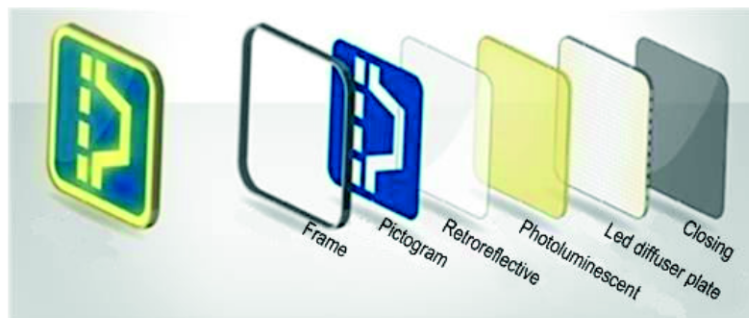
Figure 5. Signal layers scheme: pictogram, retro-reflective, photo-luminescent, and LED layers.
