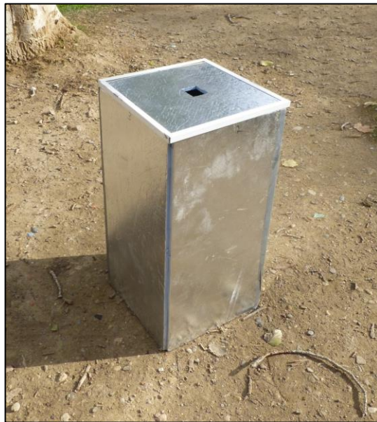
Figure 4. Box used for emissivity measurement using box method.
