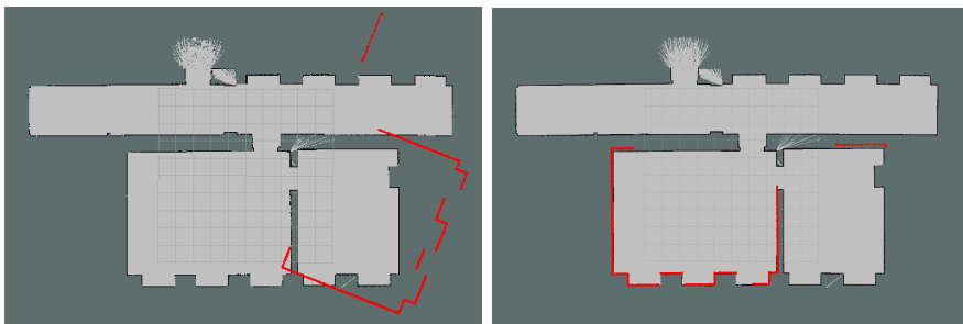
Figure 3.4: Relocalization of the robot in RViz. Red dots represent the laser data
