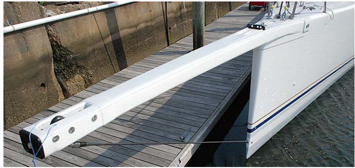
Figure 13: bowsprit adaptation in a vessel
