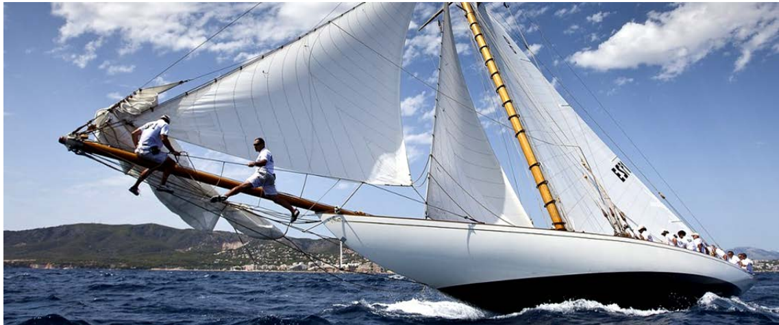
Figure 3: Classical vessel in a 2012 competition of “Classic boats”. As we can see, the bowsprit is use to provide support for all jibs.
