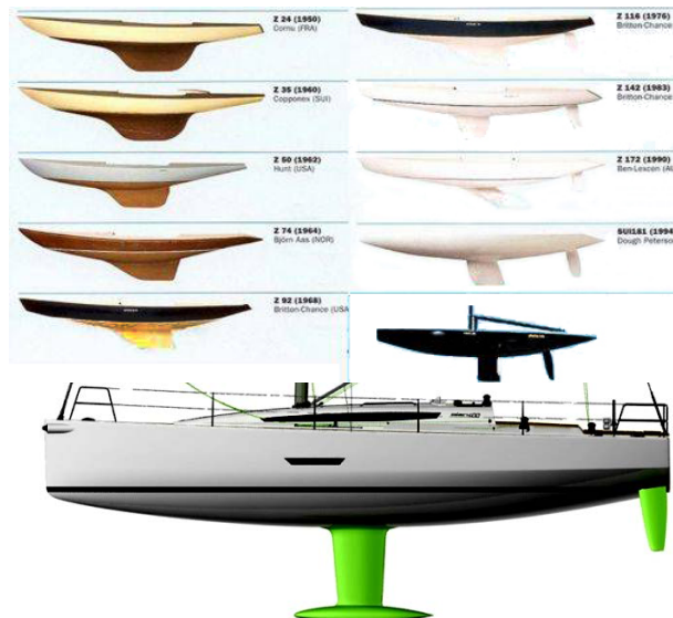
Figure 4: evolution in the shape of the boat. The picture below shows the actual configuration in most of the vessels.
