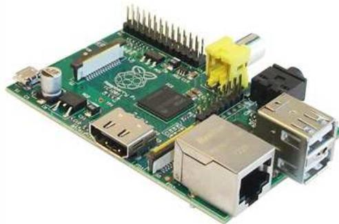
*Fig. 11 Placa Raspberry Pi B*
