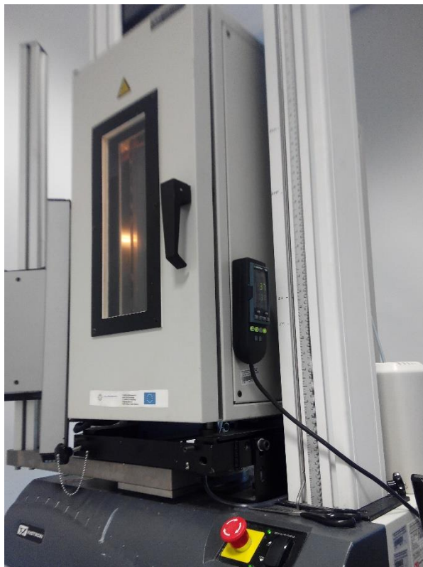
Fig. 3.12. Special heat chamber to heat all samples before and during the static tensile test at 37°C
