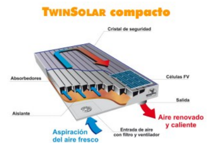
Figure 3 TwinSolar PVT air collector
