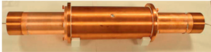
Fig. 1. ANAIS-25:D0 module: 12.5 kg mass crystal by Alpha Spectra coupled to two PMTs (Hamamatsu R12669SEL2) at the LSC clean room. Calibration window can be noticed.
