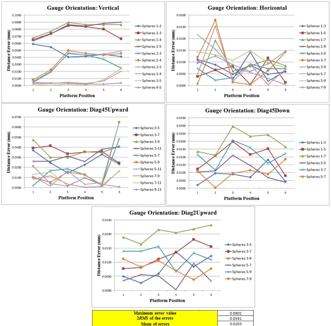
Figure 26. Maximum distance error graphs and two times the root mean square of the 252 distances between sphere centers (mm).
